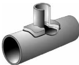
Figure C Standard Saddle/Sidewall Fusion Joint
